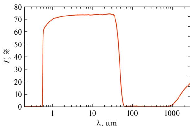
**Fig. 3.** Spectral dependence of the transmittance of the KRS-5 single crystal (thickness 2 mm).
