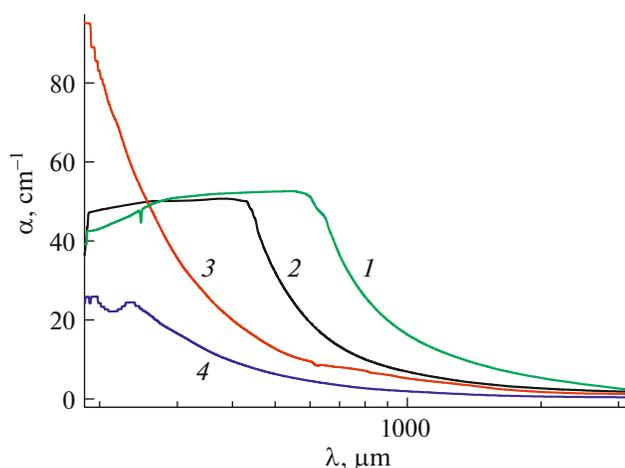
**Fig. 5.** Spectra of the attenuation coefficient in the range of 200–3000  $\mu\text{m}$  for the following single crystals: (1) KRS-5, (2) KRS-6, (3) AgCl, and (4) CsI.
