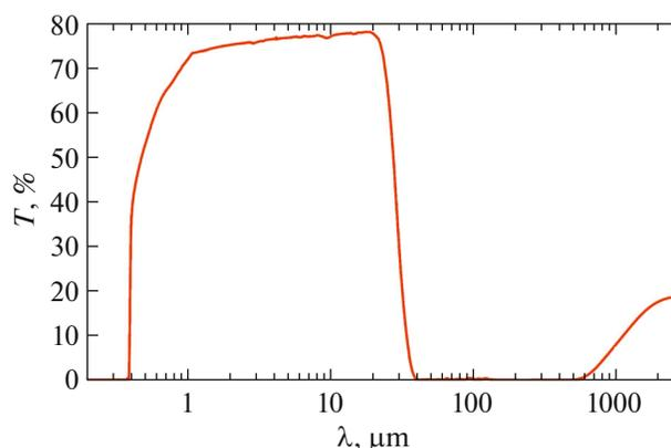
**Fig. 4.** Spectral dependence of the transmittance of the KRS-6 single crystal (thickness 2 mm).
