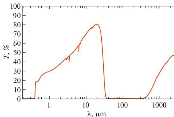
**Fig. 2.** Spectral dependence of the transmittance of the AgCl single crystal (thickness 1.16 mm, sample with poorly polished surfaces).
