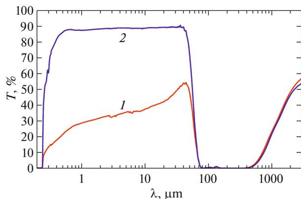
**Fig. 1.** Spectral dependences of the transmittance of the CsI single crystal: (1) sample with surface defects (thickness 4.0 mm) and (2) as-polished sample (thickness 4.2 mm).
