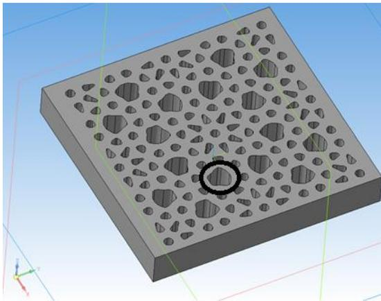
Fig. 3. An example of a 3d model of the photonic quasicrystal approximant. One of the zones with removed parts of the polymer, surrounded by a conducting region, is highlighted.
