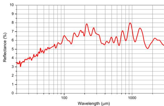
Fig. 9. Reflectance spectrum of used polymer in terahertz range
