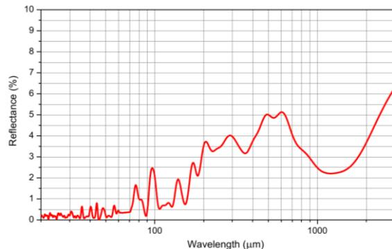
Fig. 10. Reflectance spectrum of sample with approximants of 8 order (type 1)
