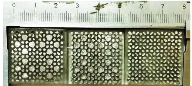
Fig. 4. Image of test photonic quasicrystals samples with different sets of approximants
