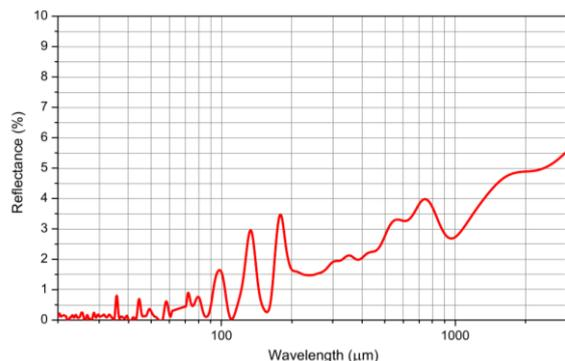
Fig. 11. Reflectance spectrum of sample with approximants of 8 order (type 2)
