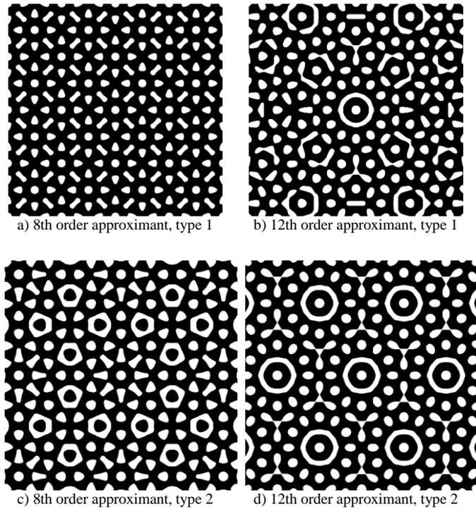
Fig. 1. Results of calculating of photonic quasicrystals approximants (black areas are filled with polymer, white areas are filled with Wood's alloy)
