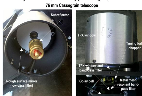
Fig. 1 – One SOLAR-T 76 mm telescope (left) has a rough surface primary to diffuse visible and near IR. Radiation is fed into the Golay cell, preceded by TPX windows, TydexBlack low-pass filter membrane, resonant metal mesh 3 and 7 THz band-pass filters, and resonant tuning fork 20 Hz chopper.
