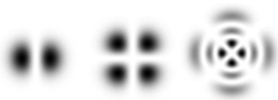
Fig. 6. Etalon intensity distributions of modes: (left) Gaussian-Hermite (0, 1), (middle) Gaussian-Hermite (1, 1), and (right) Gaussian-Laguerre (2, 2).
