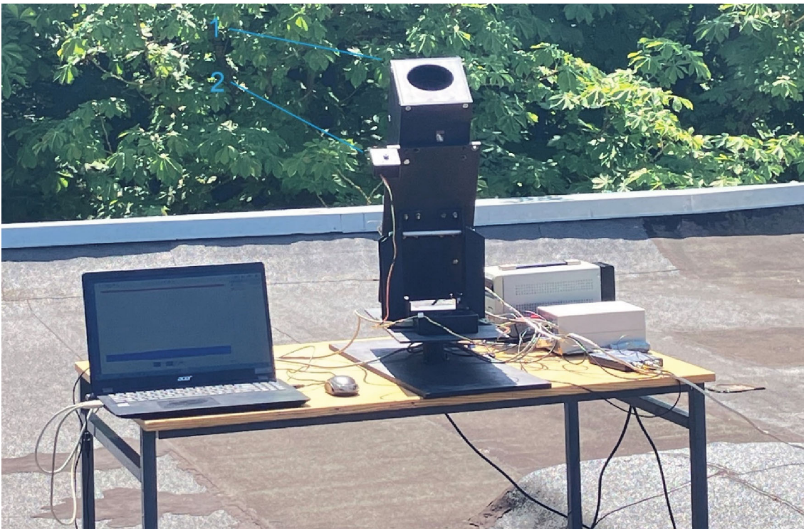
Fig. 4. The instruments to measure the background radiation of the atmosphere. They are mounted on a rotating platform: a single-channel model of the detector (1) and the sensor of clouds (2).
