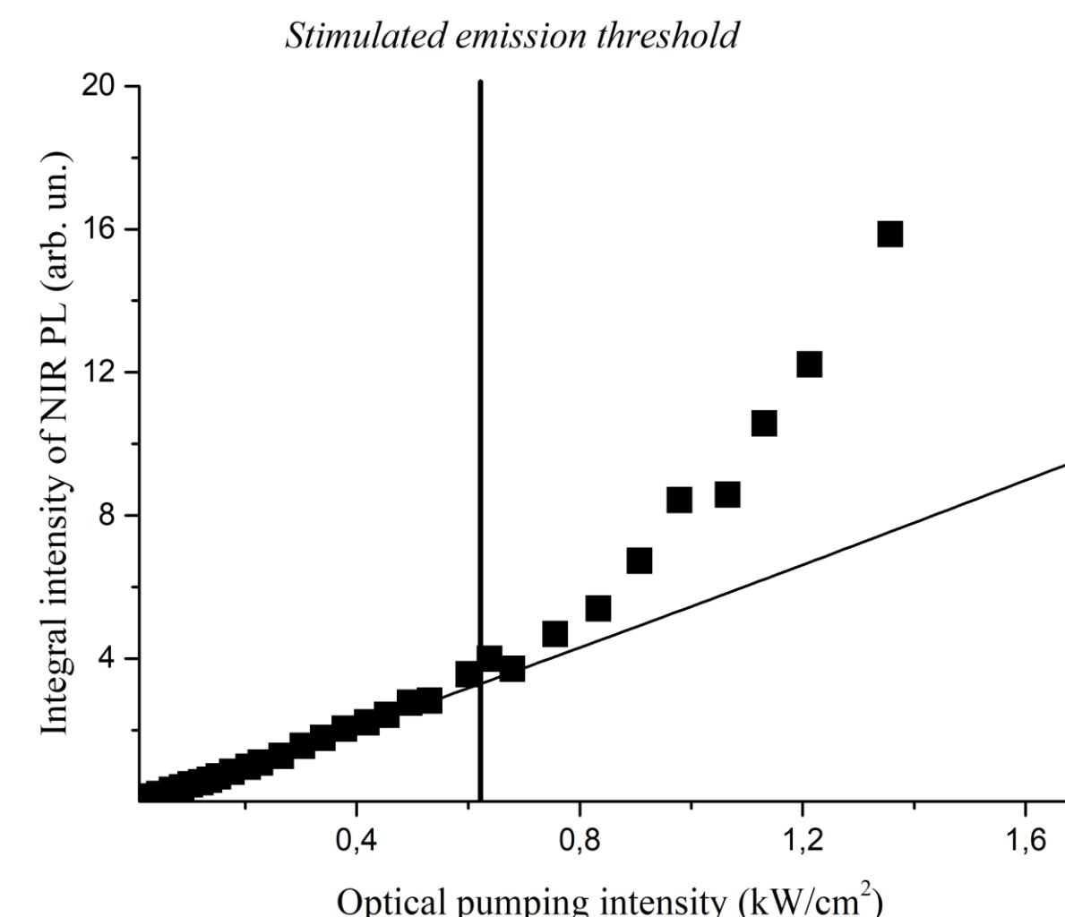
Dependence of integral intensity of terahertz photoluminescence on pump power
