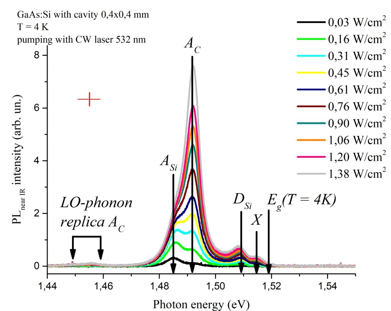
Photoluminescence spectra of the substrate in the near infrared range with CW laser pumping
