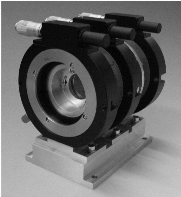
Fig. 9. Tunable wavelength polarization converter.
