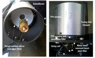
Fig. 1 – One SOLAR-T 76 mm telescope (left) has a rough surface primary to diffuse visible and near IR. Radiation is fed into the Golay cell, preceded by TPX windows, TydexBlack low-pass filter membrane, resonant metal mesh 3 and 7 THz band-pass filters, and resonant tuning fork 20 Hz chopper.
