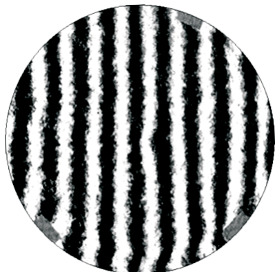
Figure 2. Typical interferometer graph of OAP mirror.
