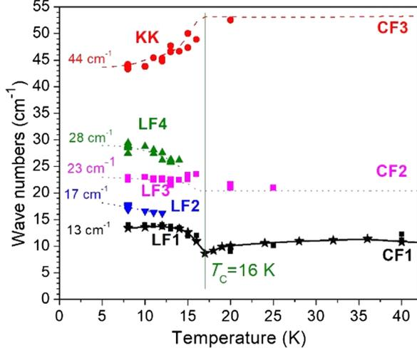
F3:1 FIG. 3. Energies of the LF, KK, and CF modes vs temperature.
