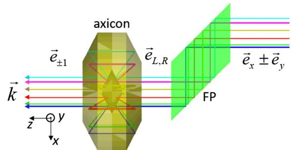
FIG. 1. Linearly polarized terahertz radiation is converted into vortex beam modes  $\vec{e}_{\perp 1}$  using a combination of a Fresnel prism (FP) and an axicon. After passing through a two-bounce FP retarder, the linearly polarized light  $\vec{e}_x \pm \vec{e}_y$  becomes circularly polarized  $\vec{e}_{L,R}$ . After passing through the axicon, the beam acquires a vortex phase  $\vec{e}_{\perp 1}$  while losing its circular polarization.
