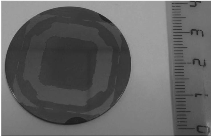
Fig. 2. Photo of the silicon substrate with the protective mask.
