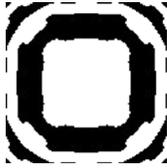
**Fig. 1.** The phase function of the focusing element (the white corresponds to phase  $\pi$ , the black—phase 0).
