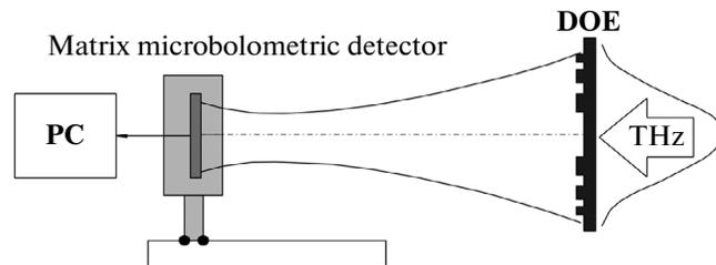
Fig. 5. The optical arrangement used in the experiments.
