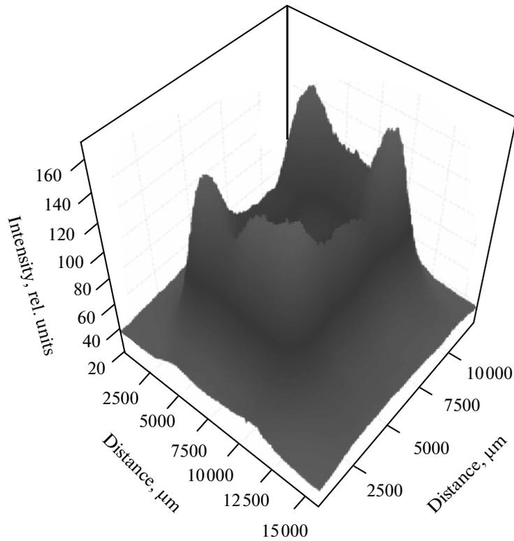
Fig. 6. Intensity distribution of THz radiation in the focal plane of the DOE.
