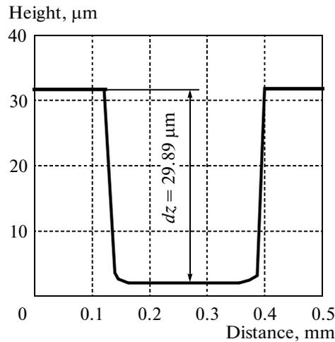
Fig. 3. The profile line of the micro relief (the arrow indicates the height).
